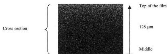
Figure 10 EDS picture of PEObr20/PEDOT semi-IPN cross section. White spots represent the sulfur domains.
